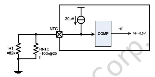
IP2726H support NTC function used for temperature detection. NTC pin output 20uA current then detect the voltage on NTC pin to determine the present temperature.
